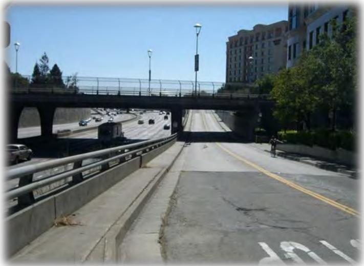
Recent modifications to 3rd Street on the east side of I-5 have added a northbound travel lane between I Street and J Street. Previously, this segment of roadway was one-way southbound. This previous configuration required motorists exiting I-5 at J Street to travel two blocks out of their way to access the I Street gateway into Old Sacramento. With the addition
